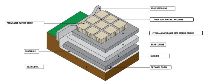
**Coverage:** 1 bag of **GATOR AQUA ROCK** will cover on average, for a 60 mm paver, 20 to 25 sq.ft. (1.86 to 2.32 meters). Super-Sack will cover on average, for a 60 mm paver, 880 to 1100 sq.ft. (81.78 to 102.2 sq. m.).
